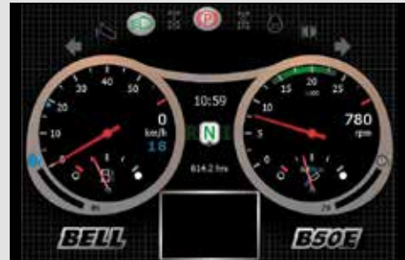
A user friendly 10" color monitor offers vital operating information, safety warnings, detailed diagnostic readings and dump body function settings.
