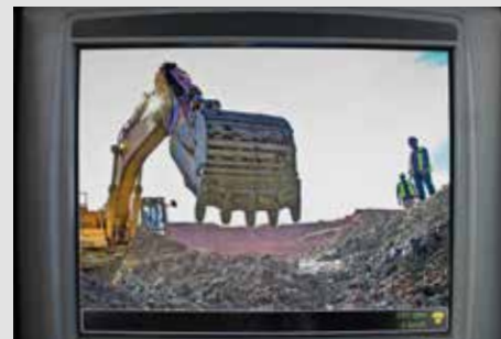
An optional integrated reverse camera and high visibility mirrors ensure superior all round visibility.
