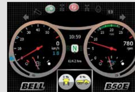
The incorporation of a pitch and roll sensor in the vehicle prevents bin operation if the truck is in an unsafe position.
