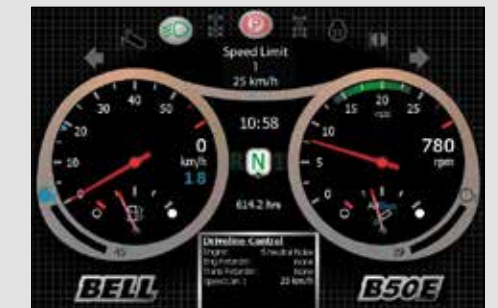
Both operator or site selectable maximum speed control allows the vehicle to automatically decelerate and apply the retarder to prevent onsite speeding.
