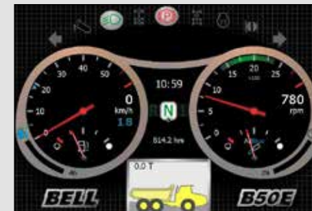
The exclusive on-board weighing presents the operator with real time information on the payload while the machine is being loaded. A 'speed restriction' mode can also be activated if the machine is significantly overloaded.
